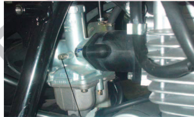
Idling speed adjusting screw
